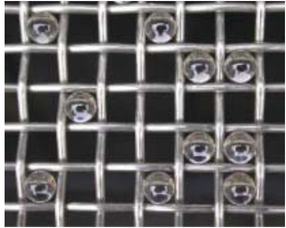
Fig. 2: Near mesh challenge particle trapped in a square mesh filter
