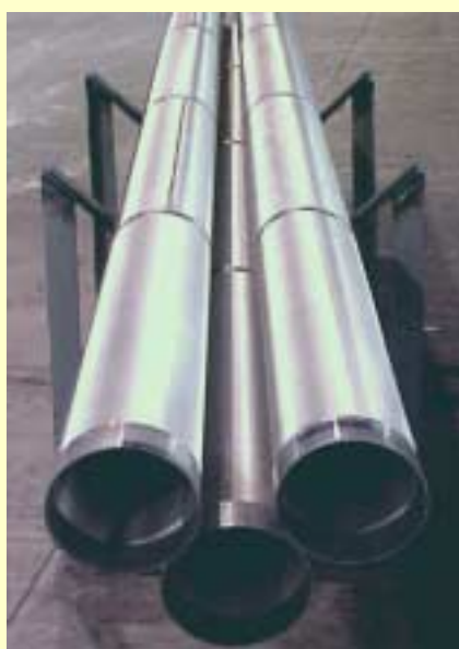
Figure 4: fabricated sand screen tubes showing weld lines
