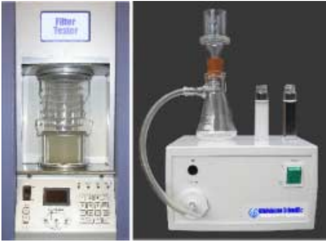
Figure 4: Challenge testing may be dry as Sonic testing or via aqueous suspensions
