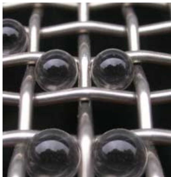
Figure 1: Challenging filter media with spherical particles gives unambiguous pore size data.
