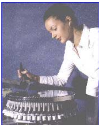
Figure 4. A 100 stage spinning riffler produces identical sub-samples
