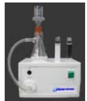
Figure 10. Clarifying a filter standard in a suspension challenge test apparatus
