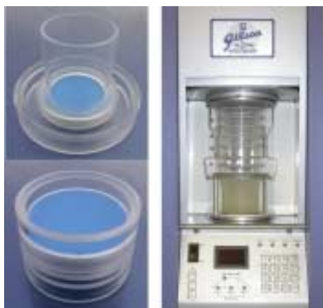
Challenge testing of filter media using the Gilsonic filter tester
