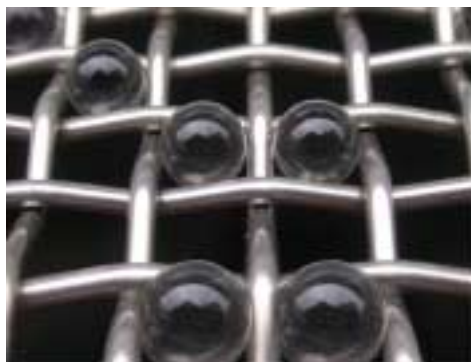
Whitehouse Scientific sieve calibration beads give NIST traceability
