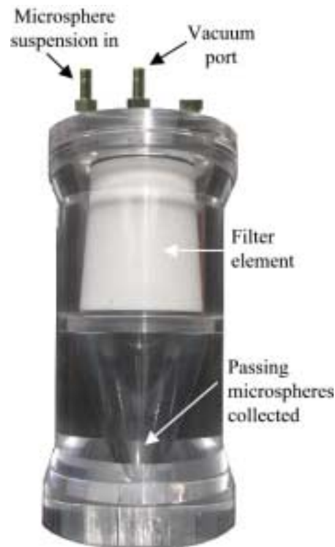
A new air filter tester revealed 140 micron pores in a nominal 5 micron filter
