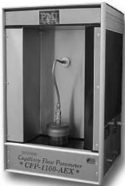
A pore size distribution instrument from PMI
