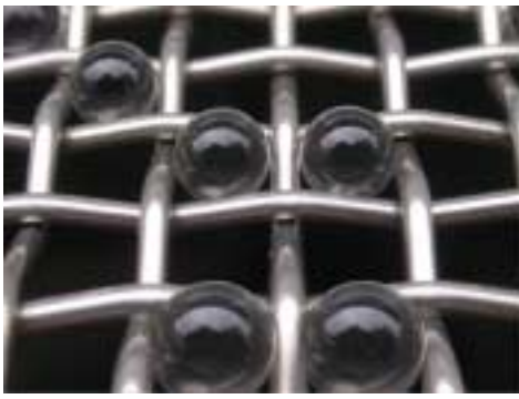
Figure 3. Glass microspheres for Sieve Calibration
