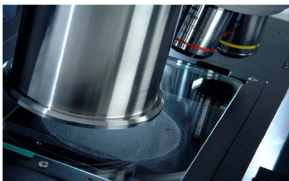
Figure 1: The powder dispenser on the Malvern Morphologi G3 particle characterisation system.
