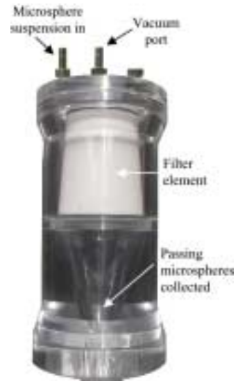
Figure 10: Challenge test apparatus for an air filter.
