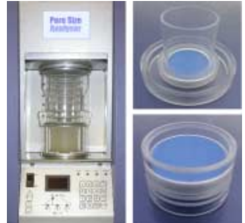
Figure 1. Sonic filter tester and sample holders
