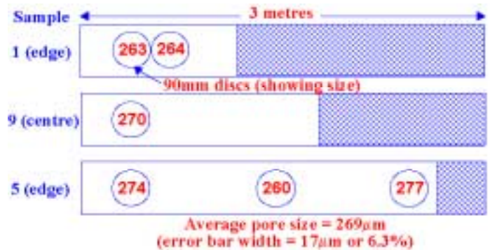
Figure 5. Measuring the uniformity of weaving
