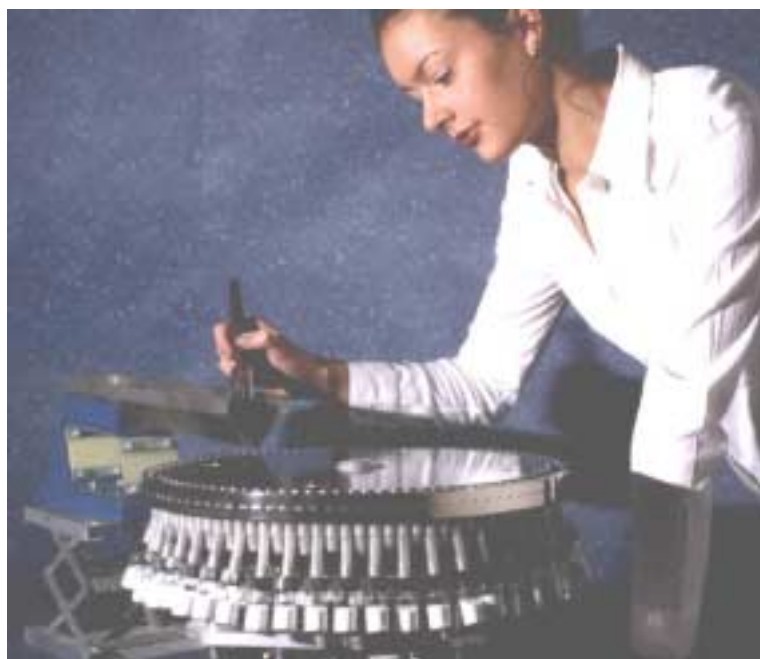
LEFT: single shot bottles of a sieve calibration standard being prepared on a spinning riffler.
