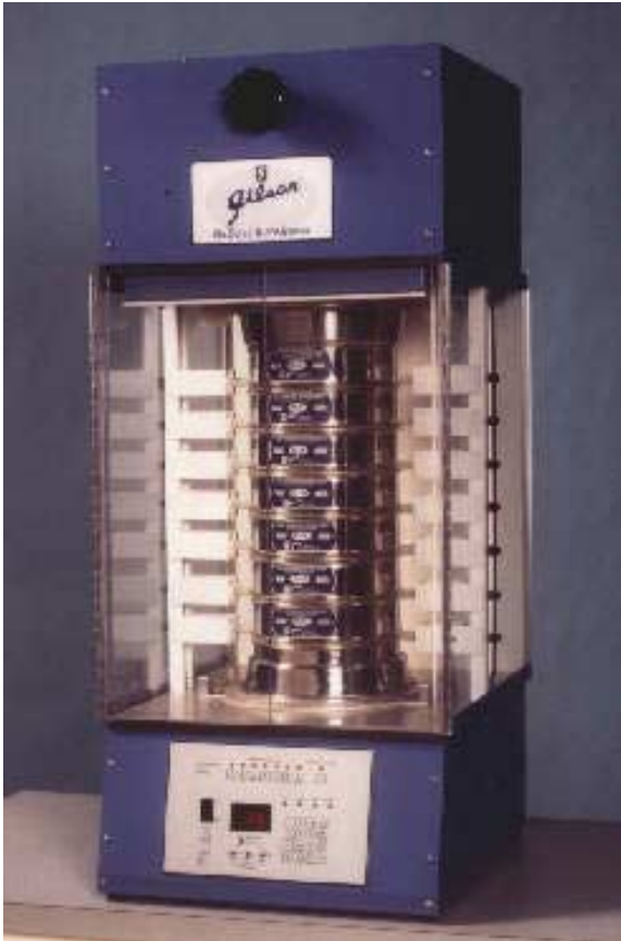
Figure 6: A Gilson Sonic Siever for 200mm diameter sieves
